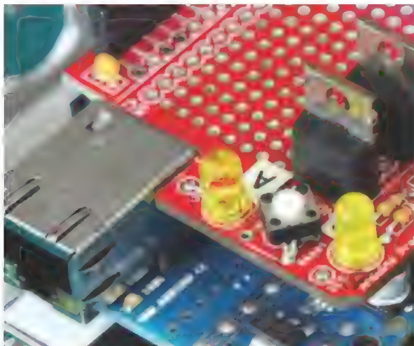
■ PHOTO 11. Close-up of SparkFun's shield. Modification done to clear the Ethernet connector.
